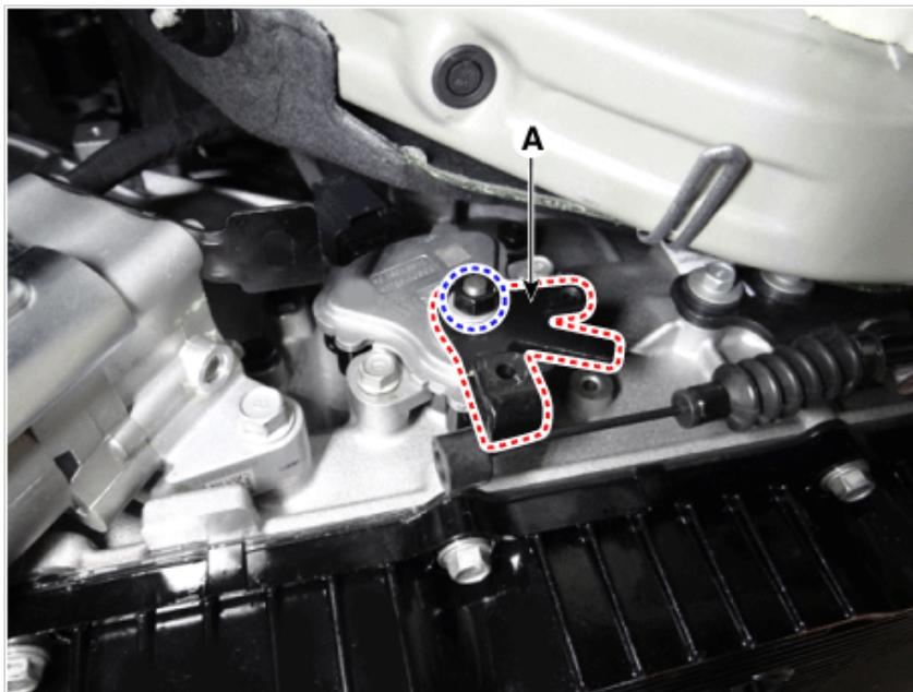
3. Remove the parking switch (A) after loosening the bolts.
