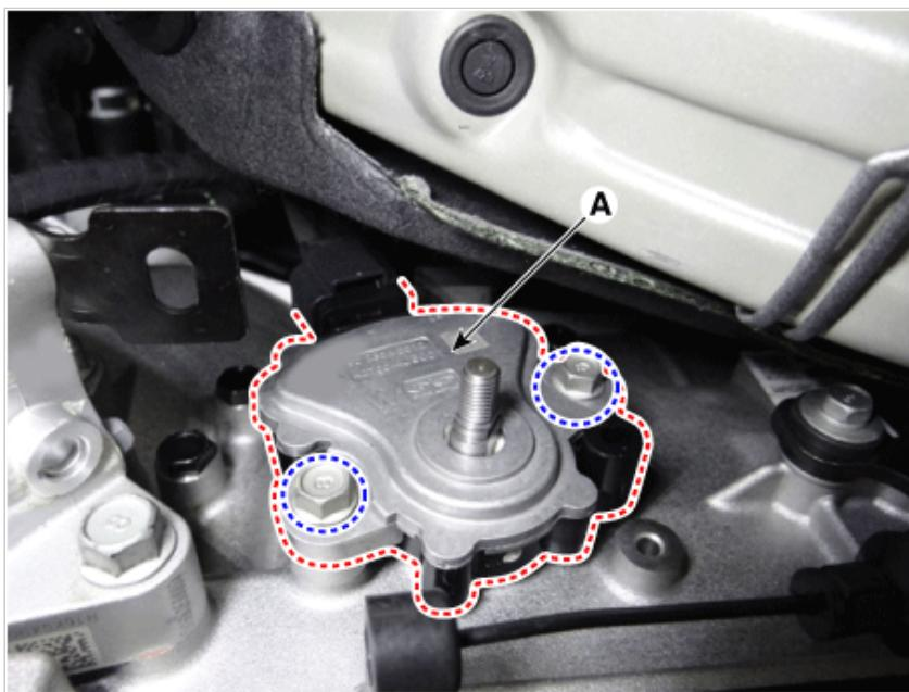
4. Disconnect the parking switch connector (A).
