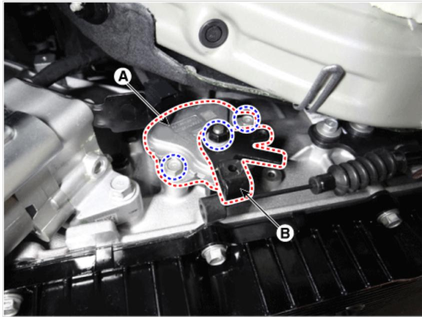
3. Align the hole in the parking release lever with the "P" position hole of the parking switch and then insert the SST parking switch guide pin (09480-D2100).
